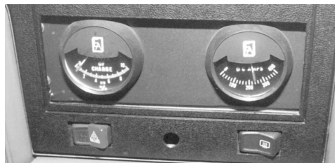
At 40 mph in 3rd gear, the ammeter reads 240A. Note that the greater load drops the needle on the state-of-charge gauge.
